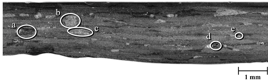
Fig. 3 Characterization of defects observed in the cross-sectional area of the composite coupons: (a) resin-rich region, (b) circular void, (c) interlaminar void, (d) complete void, and (e) micro void. The optical imaging corresponds to composite coupon 2B1 (Plate 2).
